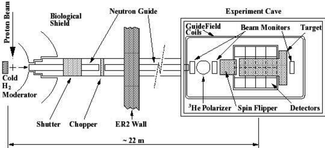
Figure 1: Layout of the  $\bar{n} + p \rightarrow d + \gamma$  experiment in FP12 at LANSCE. The setup in the FnPB at the SNS will be similar.
