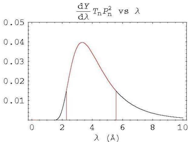
Figure 4:  $\frac{dY}{d\lambda} \times P_n^2 \times T_n$  in  $\text{n/cm}^2/\text{\AA}/\text{s}/10^9$  as a function of the neutron wavelength in  $\text{\AA}$ . The flux is from figure 3 and  $P_n$  and  $T_n$  are given in section 6. The red region defines the wavelength range of accepted neutrons in the frame.
