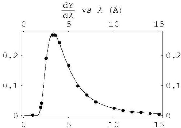
Figure 3: Predicted FnPB neutron spectrum at 1.4 MW in  $\text{n/cm}^2/\text{\AA}/\text{s}/10^9$  as a function of neutron wavelength in  $\text{\AA}$  given by Ref. [19].
