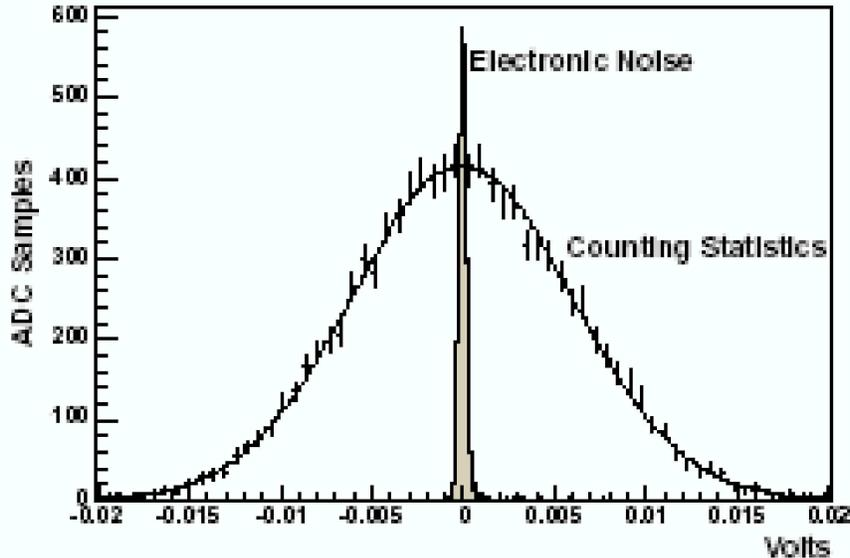
Figure 2: A typical  $\gamma$ -ray histogram from a  $B_4C$  target measured by one of the CsI detectors. For comparison an electronic noise histogram is shown.
